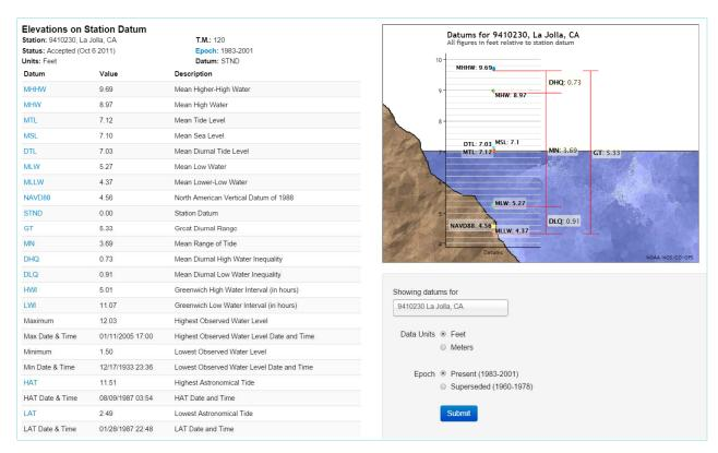
The figure to the right shows the following tidal datums referenced on 1983-2001 Epoch:
