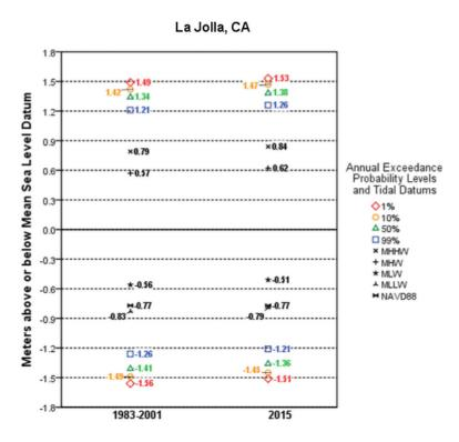
The figure above from NOAA indicates that there is a 1% chance of a tide 1.53 meters (5.0 feet), 10% change of a tide 1.47 meters (4.8 feet), 50% chance of a tide 1.38 meters (4.5 feet), and 99% chance of a tide 1.26 meters (4.1 feet) above the mean sea level datum of 2.73 feet at the La Jolla station in 2015. This is representative of potential tide fluctuations that could impact the Batiquitos, Saxony, La Costa and Leucadia Pump Stations that are located along the floodplain.
