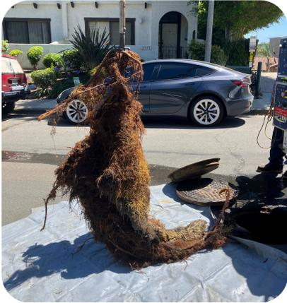
Tree roots can wreak havoc on sewer pipes, causing blockages and damage that lead to costly repairs. Recently, the LWD team discovered a tree root growing inside a sewer main line, highlighting the importance of keeping roots out of both sewer mains and homeowner laterals.
