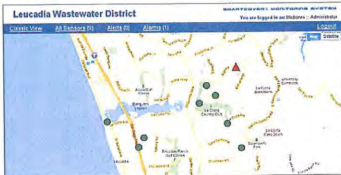
A map shows where 10 SmartCover sensors are located. One sensor shows an alarm, which could mean a potential spill in a trouble spot.
